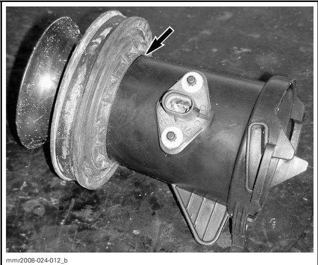
CORRECT BOOT INSTALLATION
