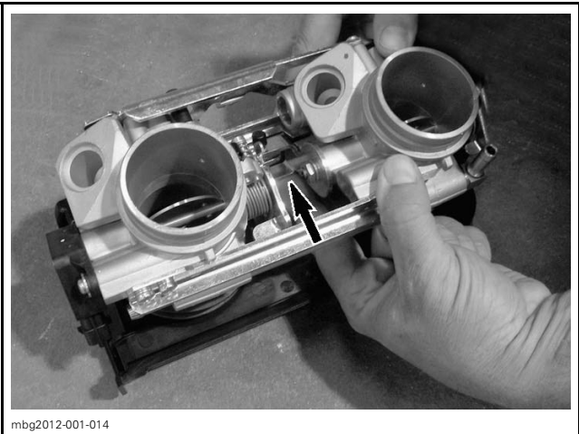
TYPICAL - PUSH TO OPEN THROTTLE PLATES
