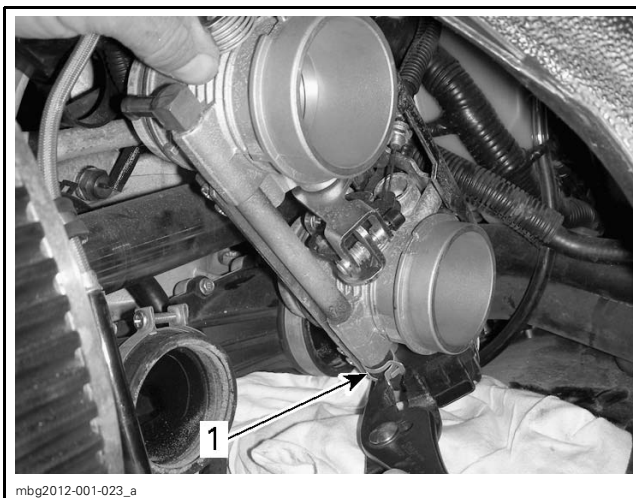
1. Coolant hose clamp to remove
